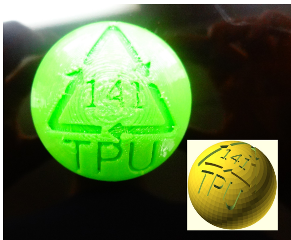
Figure 3. A toy bouncing ball was printed in thermoplastic elastomer (TPE). Inset: OpenSCAD rendering of design.
