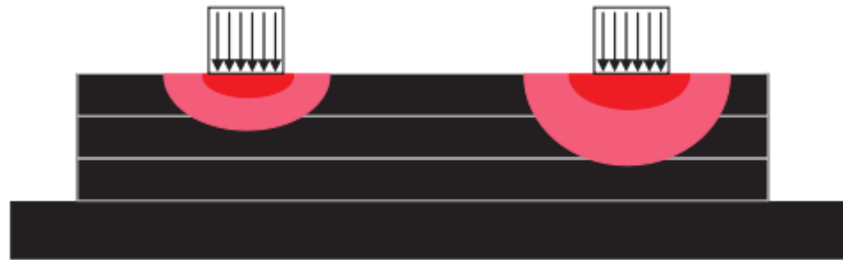
Fig. 8 Forward conduction laser welding: three black polymer layers rest on a black metal plate, arrows represent the laser, and reds represent the melt area
