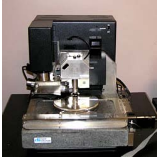
Figure 3: The Dimension 3000 atomic force microscope that was used for this test.
