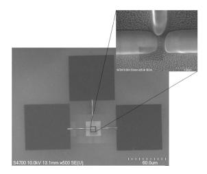
FIG. 3. SEM micrograph of the FIB deposited SET structure prior to the sputter deposition of the passivating layer. The inset in the figure shows the active area of the device; the measured device has protruding structures near the source-drain terminals.
