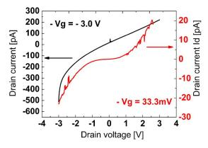
FIG. 4. (Color online) Source-drain characteristics of SET device at room temperature. Coulomb blockade is clearly visible for a lower gate bias of 33.3 mV.
