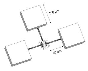
FIG. 2. Top view of the device architecture. The source and drain terminals have protruding structures near the quantum dot islands.
