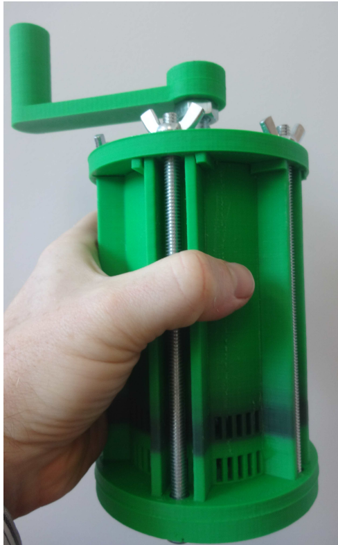
Figure 8. A 3-D printable a cassava press, which uses standard threaded rods and nuts.
