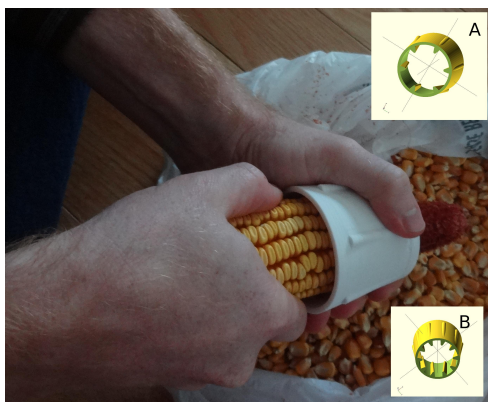
Figure 9. Corn being shelled with a 3-D printable corn sheller. Insets A and B demonstrate the ability to customize the OpenSCAD code to print corn shellers for different types of maize.
