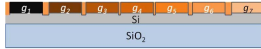
Fig. 3. Schematic depiction of Si ridge array cross section with gyrotropy ramp in cover layers.
